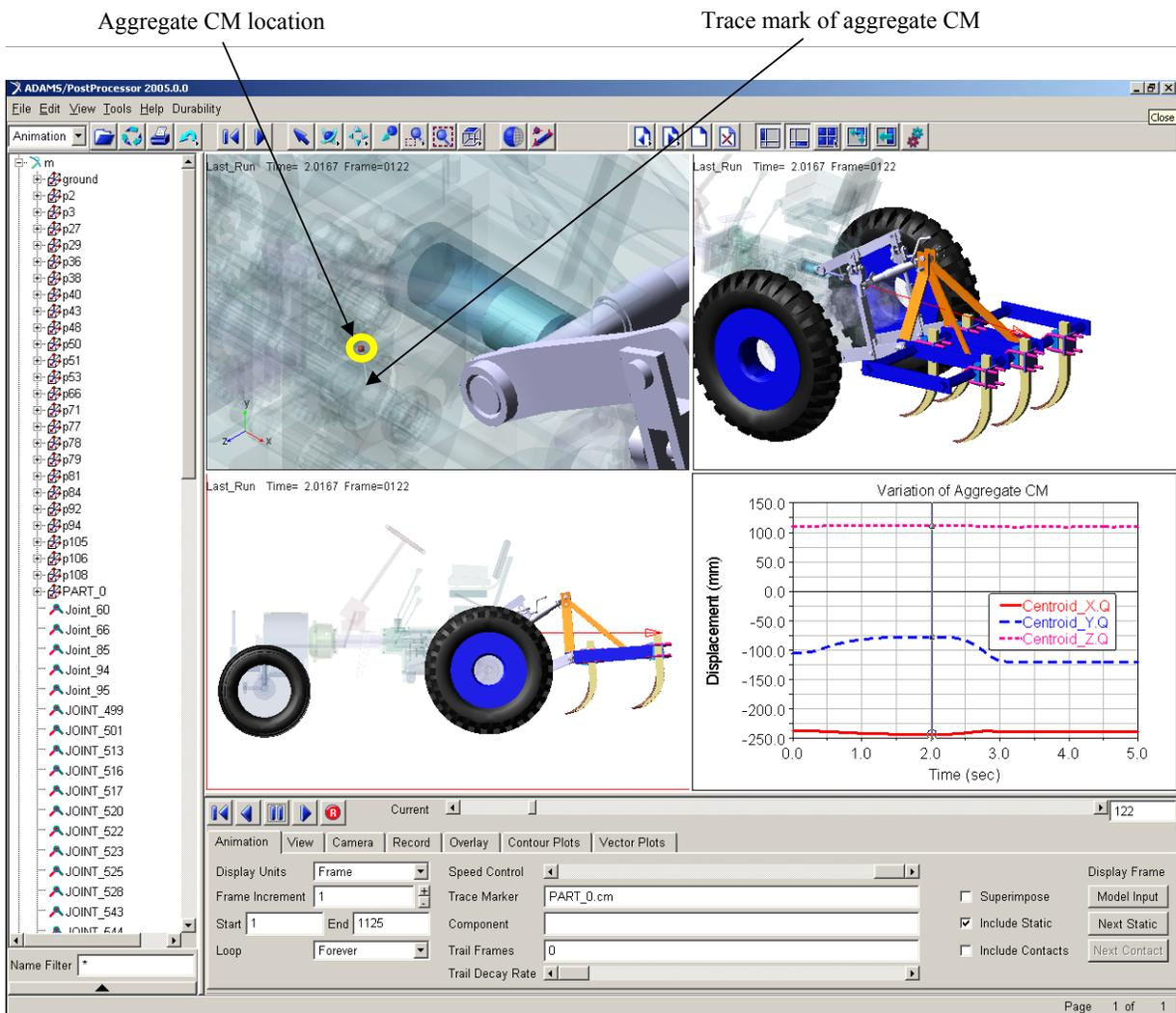
Fig. 5: Aggregate CM variation of tractor implement during simulation
