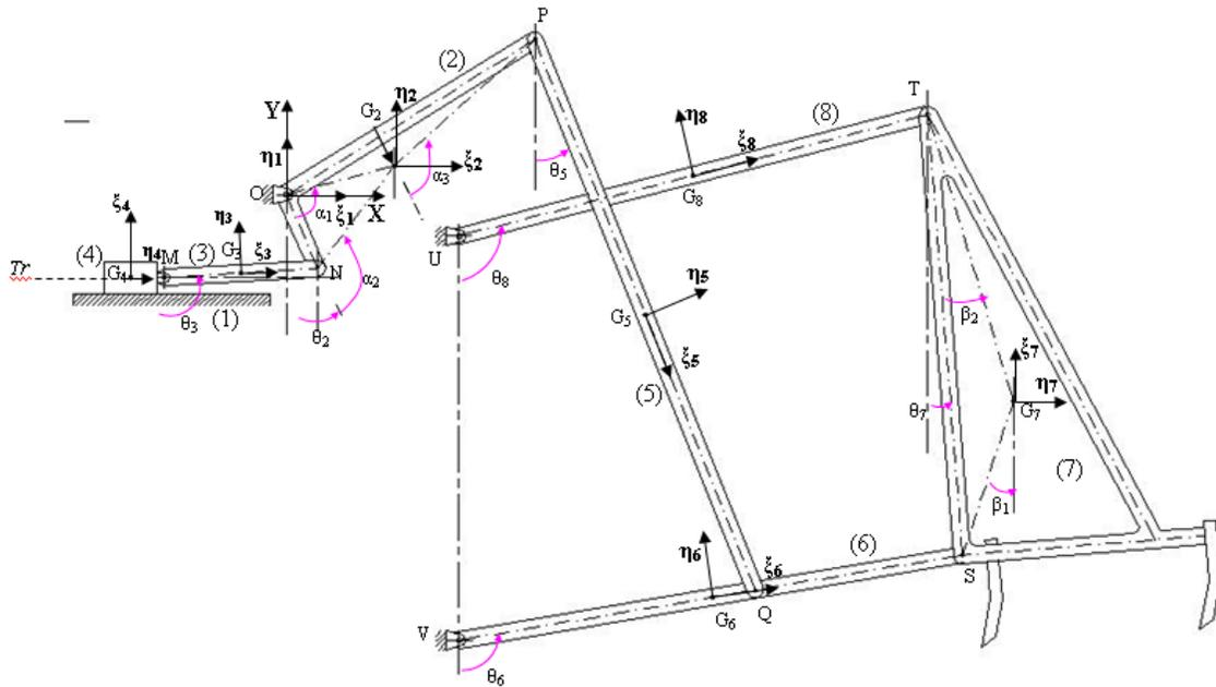
Fig. 6: Planar model of the tractor implement
