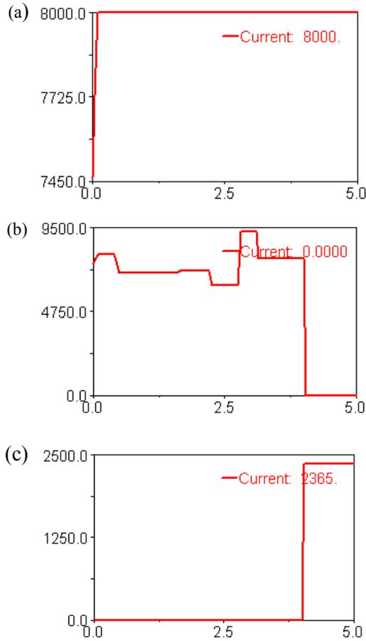
Fig. 2: STEP MATH FUNCTION (a) Constant force (b) Regulated Force: *Action Force by the piston* (c) *Reaction Force due to implement digging into the ground*:
