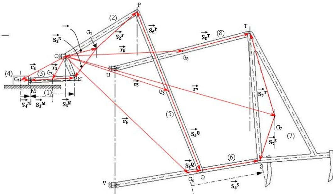
Fig. 7: Vector loops connecting different links of the tractor implement
