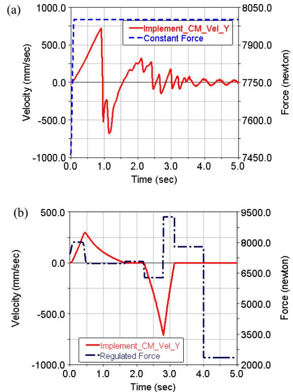
Fig. 4: Change in the velocity of the implement w.r.t time (a) actuation by constant force (b) actuation by regulated force.
