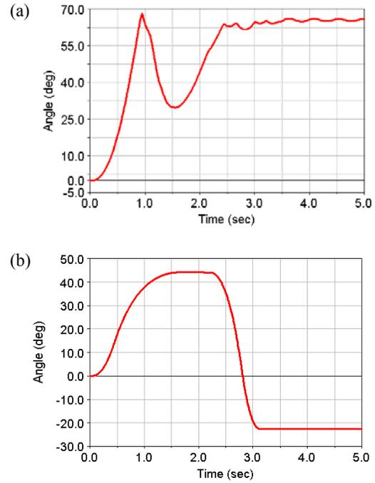
Fig. 3: Variation of connecting arm angle w.r.t Y-axis (a) actuation by constant force (b) actuation by regulated force
