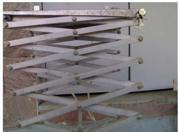
Fig.11 Fabricated scissor lift
