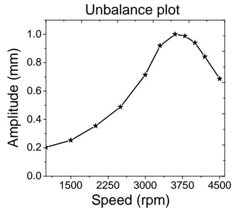
Fig. 14: Unbalance response of shaft using laser measurement
