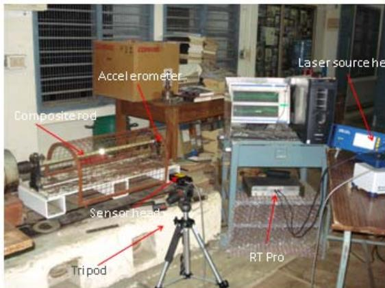
Fig. 1: The experimental setup for composite Shaft
