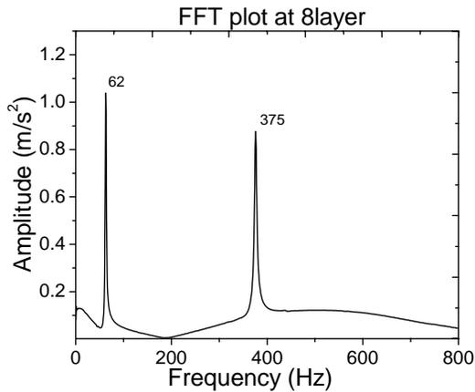
Fig. 4: FFT of accelerometer measurement for 8 layer (0-90)
