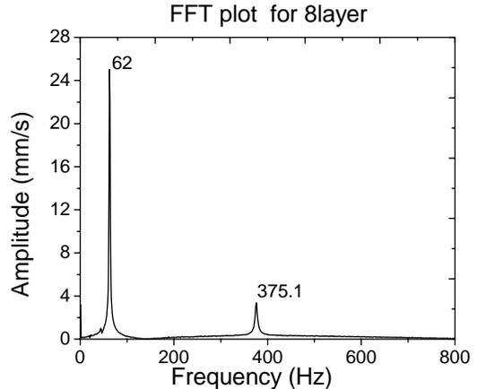
Fig. 6: FFT of Laser measurement for 8-layer (0-90)
