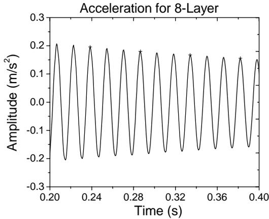
Fig. 3: Time response of accelerometer Measurement for 8-layer (0-90)
