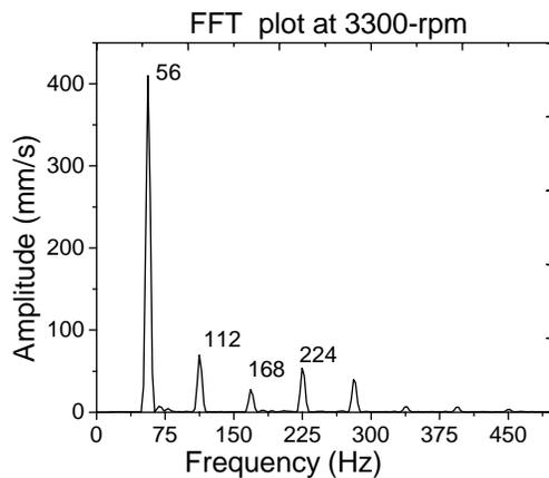
Fig. 10: FFT of Laser measurement at 3300 rpm
