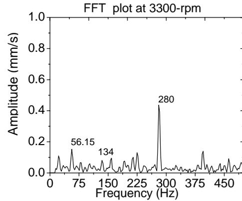
Fig. 8: FFT of accelerometer measurement at 3300 rpm
