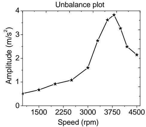
Fig. 13: Unbalance response of shaft using accelerometer measurement
