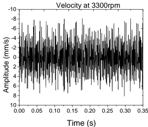
Fig. 7: Time response of integrated accelerometer Measurement at 3300 rpm
