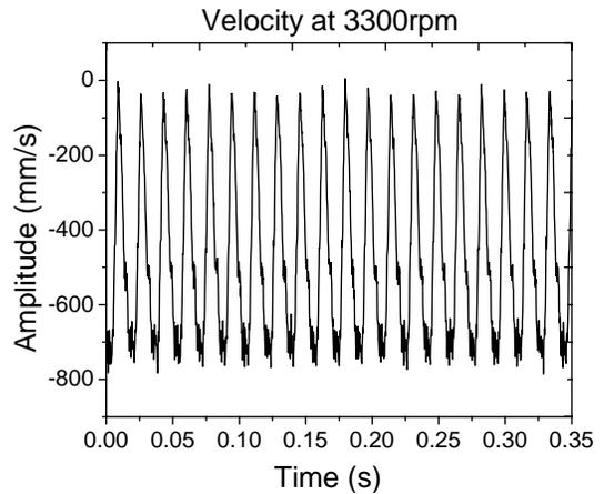
Fig. 9: Time response (velocity) of Laser measurement at 3300 rpm
