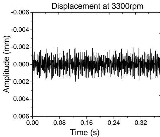
Fig. 11: Time response of integrated accelerometer Measurement at 3300 rpm
