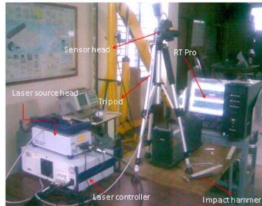
Fig. 2: The experimental setup for composite beam
