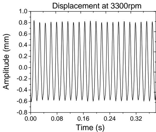
Fig. 12: Time response (displacement) of Laser measurement at 3300 rpm
