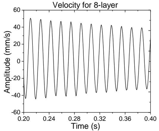
Fig. 5: Time response of Laser measurement for 8-layer (0-90)
