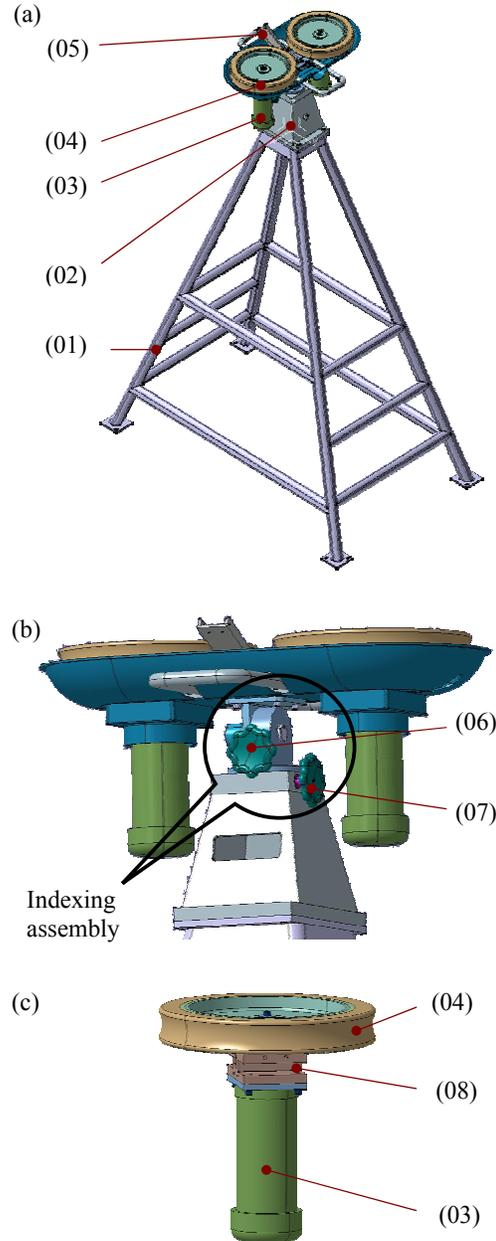
Fig.1: 3D CAD Model (a) Full Assembly, (b) Indexing Assembly (c) Wheel –motor Assembly
