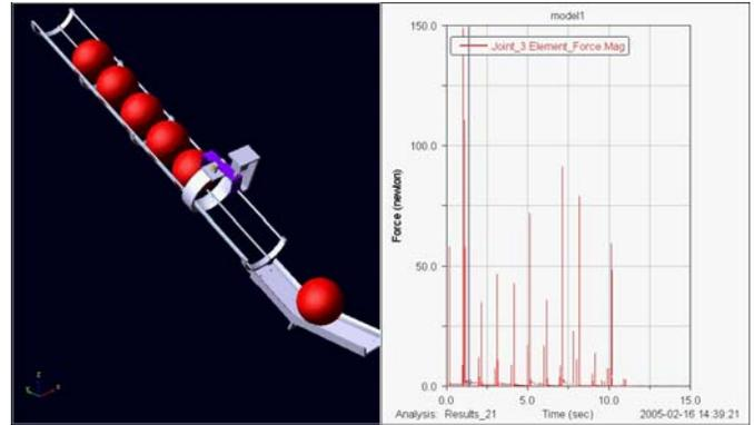
Fig.6: Simulation and synchronization of auto feeder
