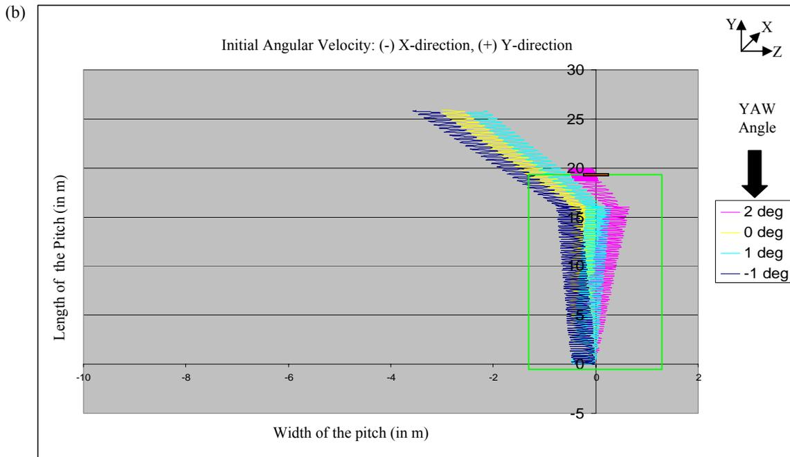
Fig 8 : Spin Bowling (a) Simulation in ADAMS (b) Ball Trajectory w.r.t. tilting of the yaw axis of the bowling machine
