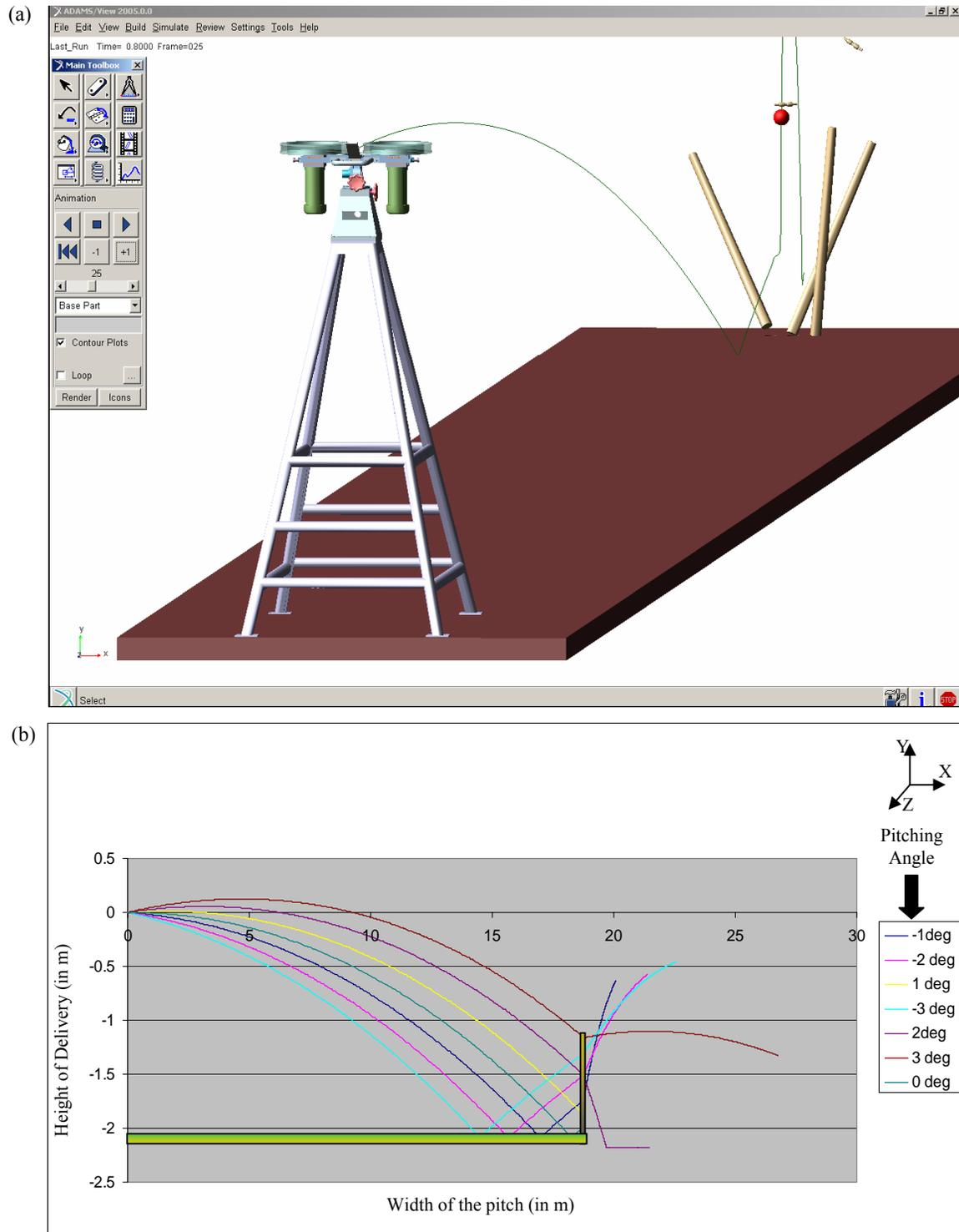
Fig 7 : Seam Bowling (a) Simulation in ADAMS (b) Ball Trajectory w.r.t. tilting of the pitching axis of the bowling machine
