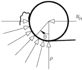
Fig. 9: Pressure profile on end-effector roller
