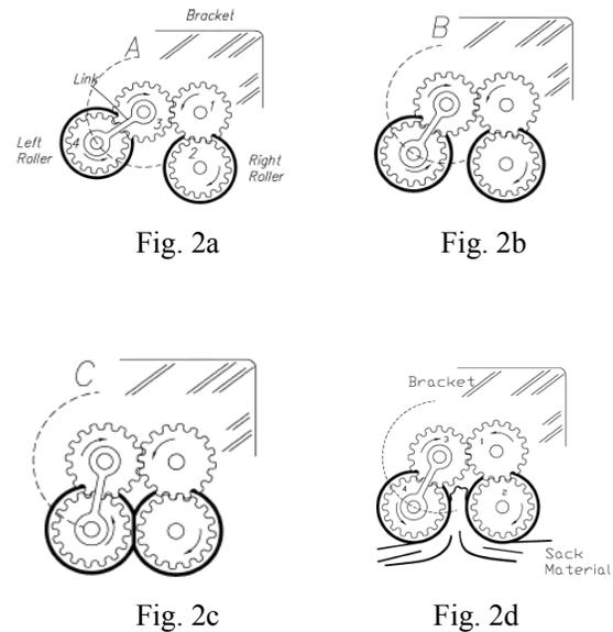
Fig. 2: End Effector Mechanism
