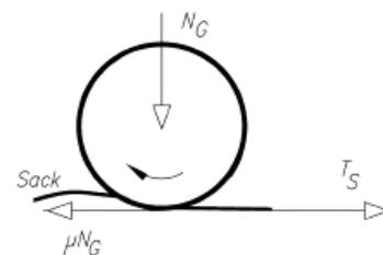
Fig. 8: Force acting on the roller
