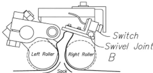
Fig. 7: Switch Location for Signal
