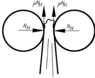
Fig. 10: Friction forces prevent the sacks from sliding
